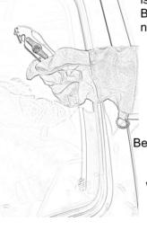
The Belt Cutter has an extra sharp blade for cutting belts. Belts should be tensioned using one hand to facilitate cutting. After that, using your other hand, position the belt cutter using the guidance groove to align the angle with the belt's edge, after which pulling will near effortlessly cut the Belt.
